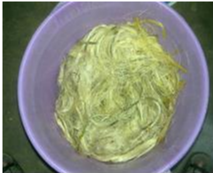
Fig.8 Fibre dried in oven for 6Hrs
