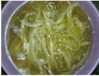
Fig.7 Fibre dipped in NaOH
